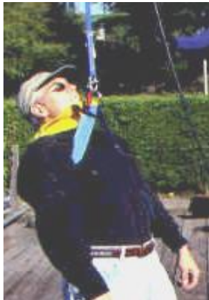
Static Test showing how the attachment point on the Forespar Passagemaker Harness comes close to the face. This also manifested itself during the in the water testing.
