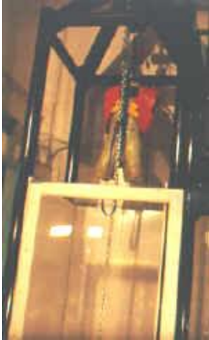
Harness ready to be dropped in the Dynamic Load Test Fixture.
