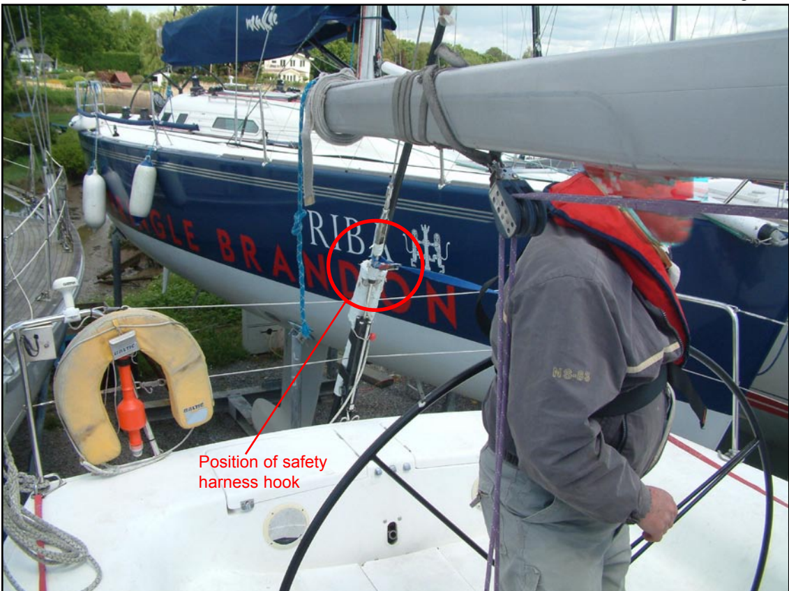
Position of day skipper's safety harness on rod backstay
