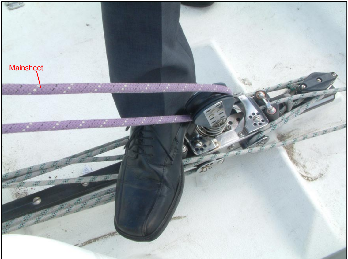
Day skipper's leg position on the traveller rig
