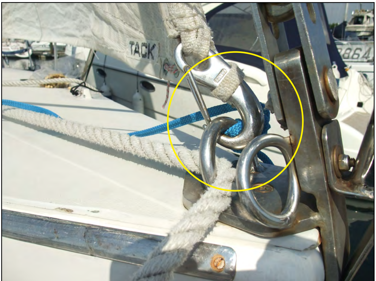
Figure 4: Genoa tack connected to the forward pad eye
