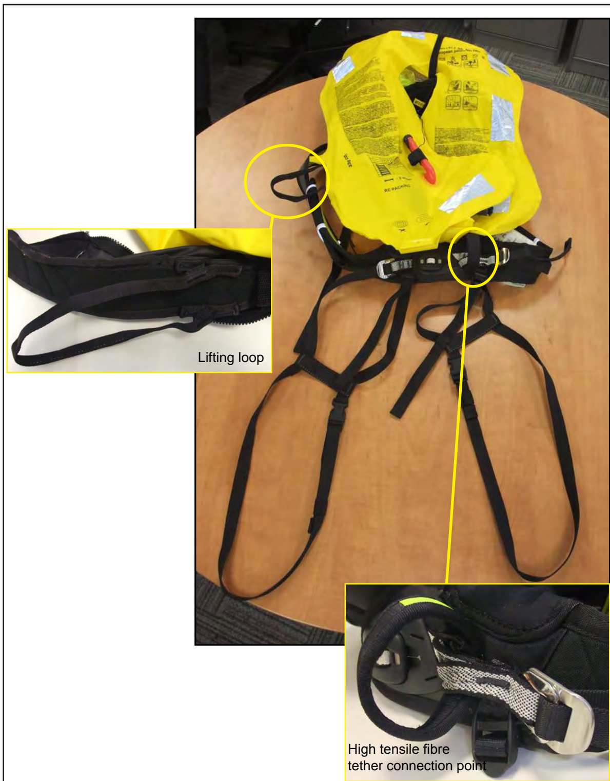
Figure 12: Skipper's Spinlock Deckvest 150 Pro Sensor lifejacket, harness and thigh straps
