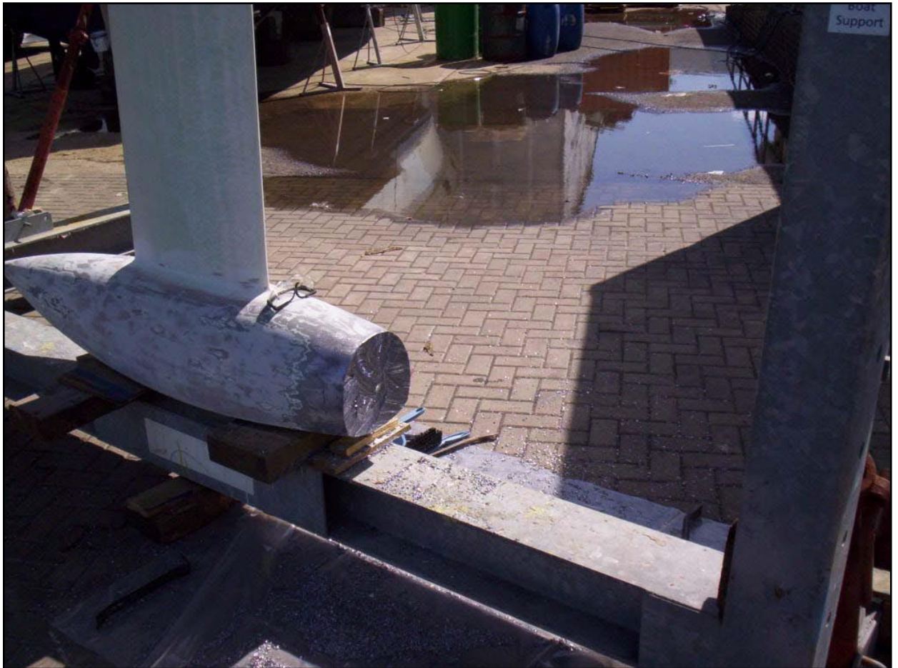
Face of the removed section from the front of the fin bulb
