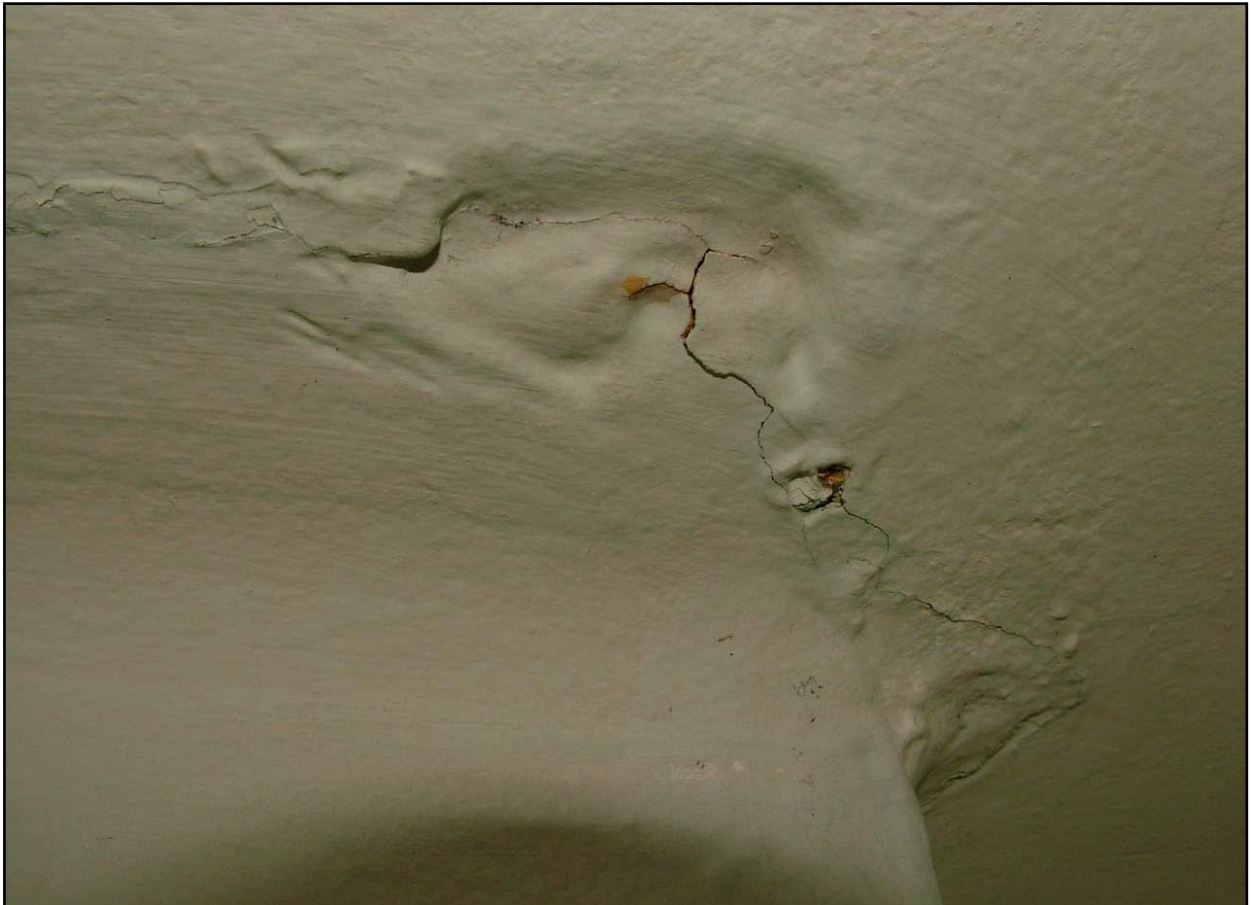
Keel of Guts "n" Glory showing cracking of the epoxy filler and anti-fouling
