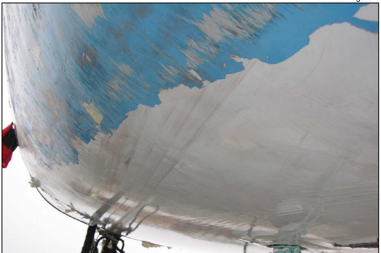
Paint and scratch marks on starboard side
