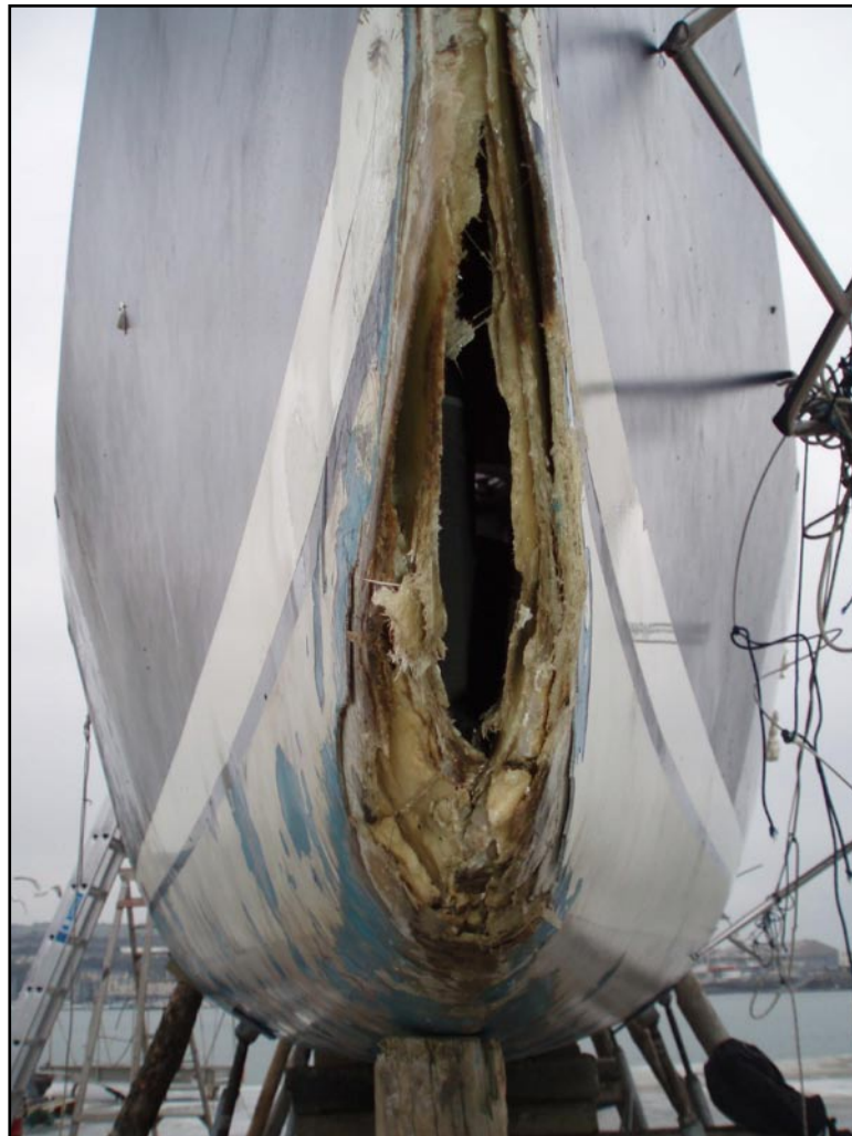
Stem damage showing full penetration of the hull
