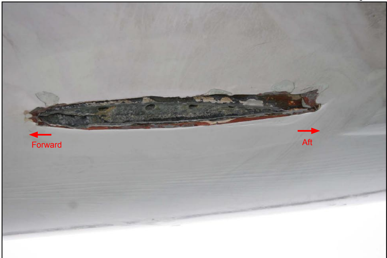
Remains of fin, showing point of detachment
