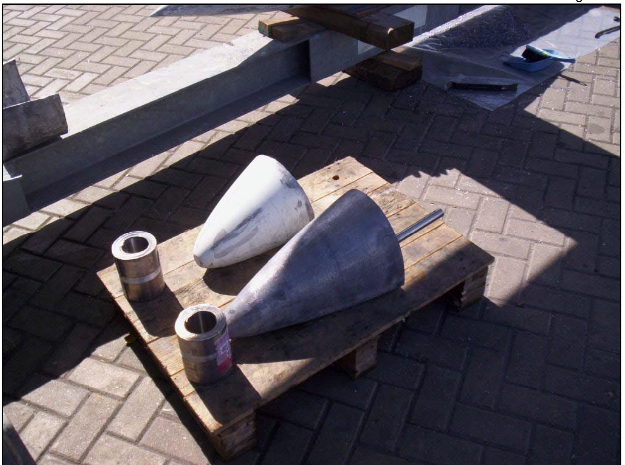
Removed and new section of bulb, lead sheeting and stainless steel fixing pins
