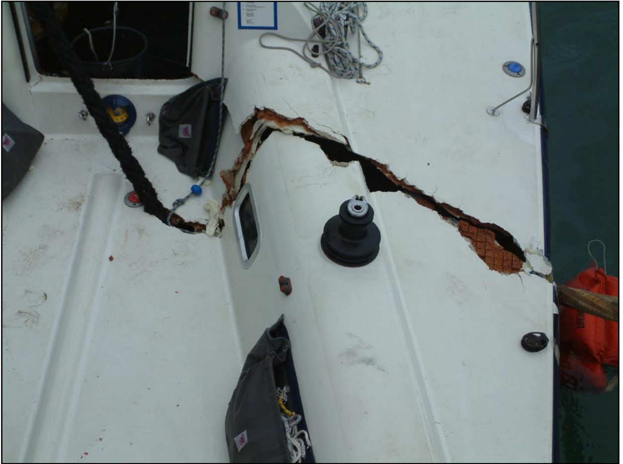
Rope damage - starboard side of cockpit
